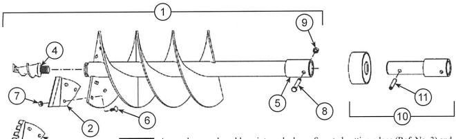
Augers have replaceable points and edges. Serrated cutting edges (Ref. No. 3) and optional points (Ref. No. 12 and Ref. No. 13) are available to aid penetration in tough digging conditions. Flights are replaceable except on 4" and 6", where the flight is a continuous spiral. Cutting edges on 4" and 6" augers are welded on the auger.
